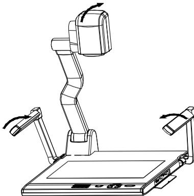
2. Carefully **fold** the camera stand down to the front panel.
