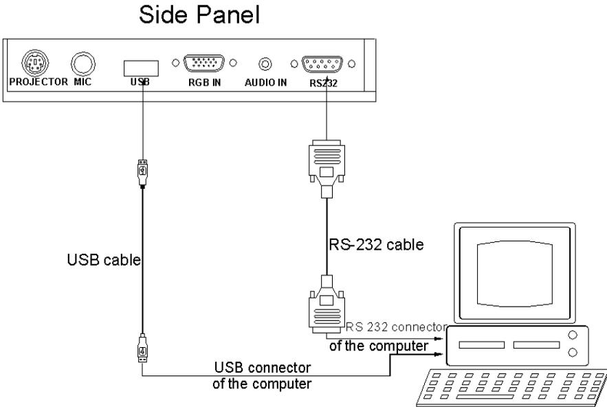
Use the computer RS232 cable (9-pin to 9-pin) to make the connections displayed below to control the visualizer from an external computer.
