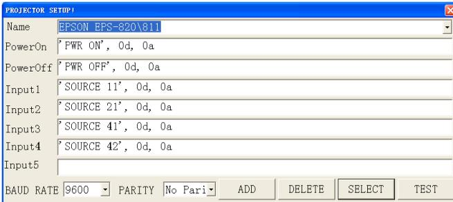
Connect the visualizer to a computer with a RS232 cable (Please disconnect the projector from the RS232 port first) and select the Baud Rate and Parity based on the projector's Baud Rate, then click the "TEST" button to pop up the Projector Code Test dialog box, input the Baud Rate and Parity based on the projector's Baud rate, then click "Open".
