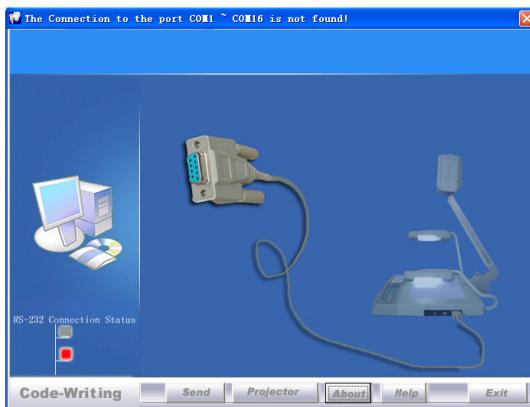
When the indicator of “Current RS-232 Connection Status” is green, that means the connection between the visualizer and the computer’s RS232 connector is good. If the indicator is red, please check if the RS232 cable is connected correctly. When all the cables are connected correctly, please click “Projector” to select your projector model under the drop-down list, then click “Send”. If you can not find your particular projector model in the “Projector”, please do the following:
