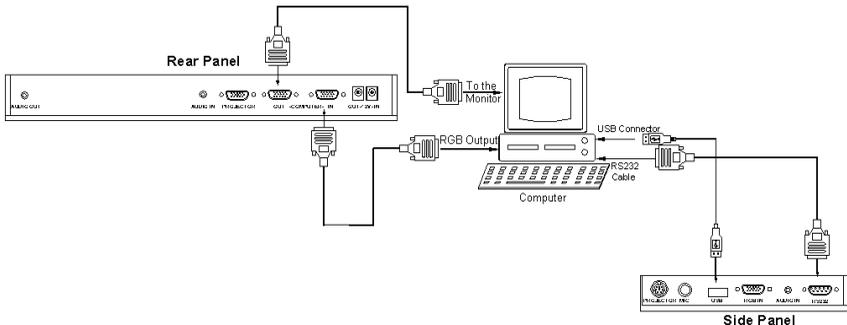
**Note:** You can connect a laptop computer to the RGB IN port of side panel using a RGB cable.
