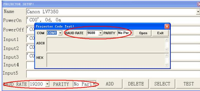
Click the projector control buttons on the visualizer's operating panel to check if the control code that the program received is the same as the sending code. If the receiving code is same to the sending code, the input codes are correct. If the visualizer can not control the projector, please do the following.
